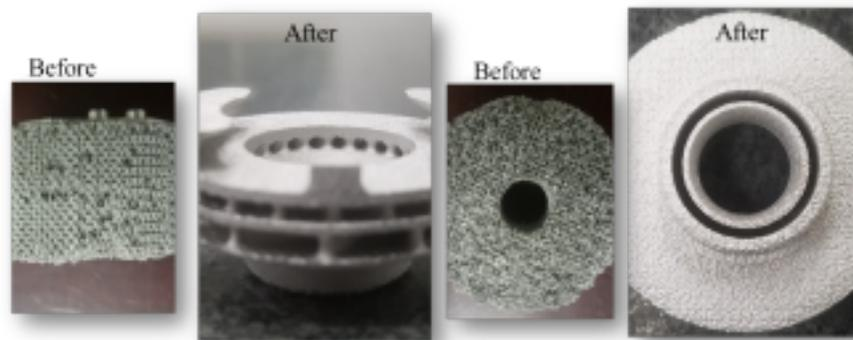
This first example shows a printed Inconel 718 mesh structure with lattice support both internal and external. The part pictured measures roughly 1 ½ inch in diameter by 1 inch in height. This was a proof of concept used to determine post-processing effectiveness and removal depth.
