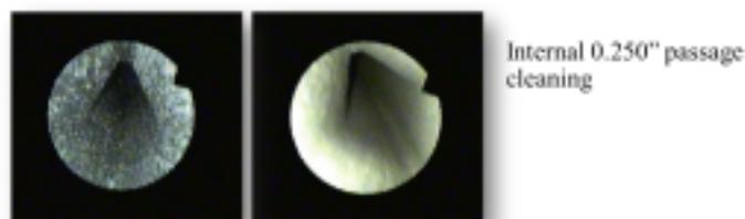
It should be noted, however, that for long and thin passageways, with a length to diameter ratio of in excess of approximately 25:1, mechanical flow of solution through the passages are required to maintain a consistent concentration of reactants and permit the removal of reactant byproducts.
